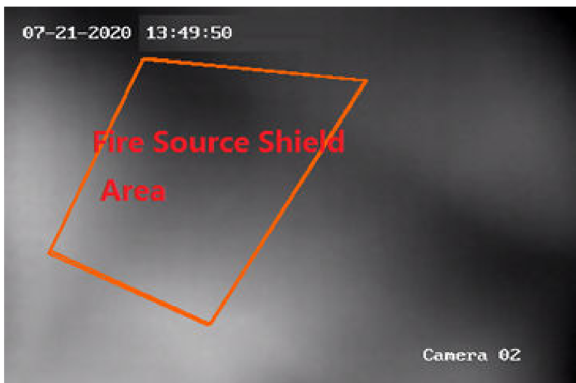
Figure 5-9 Fire Source Shield Area
